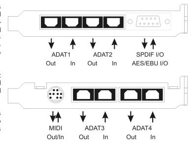
The included **MIDI** breakout cable is connected to the 9-pin **Mini-DIN** connector, providing **two MIDI** inputs and outputs.
