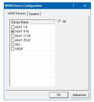
The screenshot to the left shows the multichannel WDM devices available with the HDSPe RayDAT after selecting 'Multi-Channel' in the WDM Devices listbox and hitting WDM Configure. In this example the device ADAT 9 to 16 is active.
