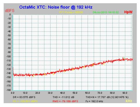
As can be seen in the above picture, the noise floor stays fully unchanged up to 30 kHz. With sample rates up to 96 kHz the noise shaping happens outside of the transmission range.
