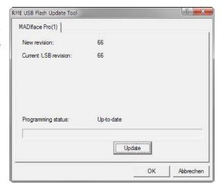
When the update unexpectedly fails (status: failure), the unit's Safety BIOS will be used from the next boot on, the unit stays fully functional. The flash process should then be tried again.
