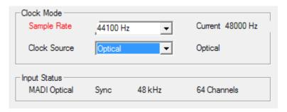
text label signals the error condition, and prompts the user to set 48000 Hz manually as sample rate. Under ASIO the audio software sets the sample rate, so that such an error can not happen. If the input sample rate is different then there will be no Sync indication.
