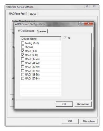
The screenshot to the left shows the multi-channel WDM devices available with the MADIface Pro after selecting 'Multi-Channel' in the WDM Devices listbox and hitting WDM Configure. In this example the devices MADI 1 to 8 and MADI 9 to 16 are active.
