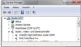
Windows does not support USB Audio 2.0 directly. The MADIface Pro will be detected when in CC mode, but automatic driver installation will fail.
