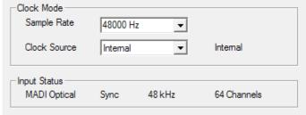
This way, configuring any suitable audio application for digital recording is simple. After connection the MADIface Pro displays the current and external sample frequency. This parameter can then be changed in the application's audio attributes (or similar) dialog.
