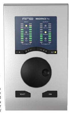
The button **DIM** is also used for **Recall**, to load a specific listening volume for the Main Out that can be defined in TotalMix FX. Pushing the knob SET for 2 seconds when OUT is selected stores the current setting. If the volume (output level) had been changed pressing DIM for two seconds will restore the former value.
