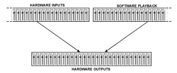
TotalMix can be used in the above view (View Options **2 Rows**). However, the default is a vertical alignment in three rows as known from an Inline desk, so that the row *Software Playback* equals the *Tape Return* of a real mixing desk:
