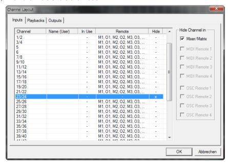
In the above example channel 23/24 have been made invisible. If these are not used this is an easy way to remove them from the mixer completely.
