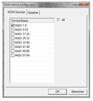
The screenshot to the left shows the multichannel WDM devices available with the MADIface USB after selecting 'Multi-Channel' in the WDM Devices listbox and hitting WDM Configure. In this example the device MADI 1 to 8 is active.
