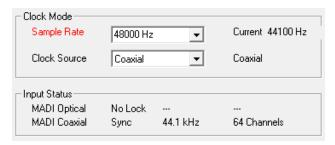
Under ASIO the audio software sets the sample rate, so that such an error can not happen. If the input sample rate is different then there will be no *Sync* indication.
