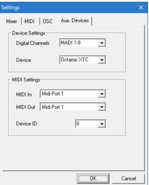
When using more than one OctaMic XTC these must have different Device IDs (configuration is done at the OctaMic XTC). *Aux Devices* supports to set different Device IDs to the 8-channel blocks as well. Storing the setting is done automatically when selecting a Device ID. To check the current assignments select all 8-channel blocks sequentially.
