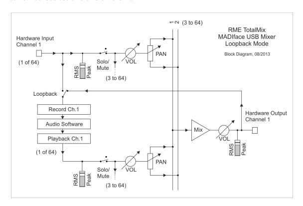
As each of the 32 stereo hardware outputs can be routed to the record software, and none of these hardware inputs get lost, TotalMix offers an overall flexibility and performance not rivalled by any other solution.
