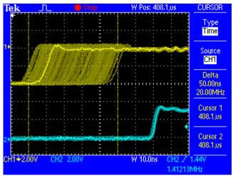
The cleaned and jitter-freed signal can be used as reference clock for any application, without any problem. The signal processed by SteadyClock is of course not only used internally, but also available at the units word clock output. It is also used to clock the digital outputs MADI and ADAT.
