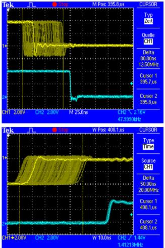
The cleaned and jitter-freed signal can be used as reference clock for any application, without any problem. The signal processed by SteadyClock is of course not only used internally, but also available at the units word clock output. It is also used to clock the digital outputs MADI and ADAT.
