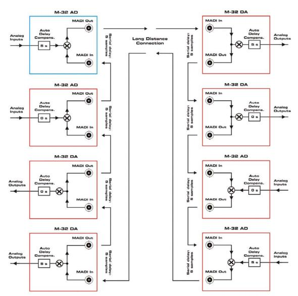
Despite serial cabling the playback is sample accurate between all units, because the converters automatically activate *Delay Compensation*.
