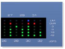
**METER PH** provides a Peak Hold function, either permanently (**ON**) or switched off by Auto Reset (**AR**) after 3 seconds.
