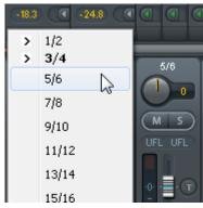
**Trim Gain.** After a click on the **T**-button one channel's faders are all synchronized. Instead of changing only a single routing the fader affects all the channel's active routings. For a better overview the faders currently not visible are indicated by orange triangles beside the fader path. When moving the fader the triangles also move to a new position, equalling the faders new settings.
