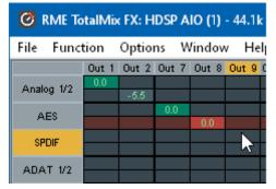
To maintain overview when the window size has been reduced, the labels are floating. They won't leave the visible area when scrolling. A right mouse click on the labels brings up the context menu with the exact same options as in the mixer view: Copy / Mirror / Paste /Clear input channels and submixes.
