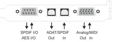
The **ADAT** I/O can also be used as **optical SPDIF** I/O, if set up accordingly in the Settings dialog.
