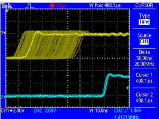
The screenshot shows an extremely jittery SPDIF signal of about 50 ns jitter (top graph, yellow). SteadyClock turns this signal into a clock with less than 1 ns jitter (lower graph, blue). The signal processed by SteadyClock is of course not only used internally, but also used to clock the digital outputs. Therefore the refreshed and jitter-cleaned signal can be used as reference clock without hesitation.
