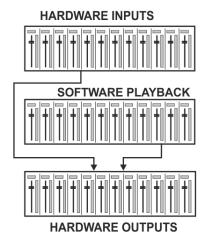
Click on the Hardware Output channel in the third row where the audio signal is supposed to show up. This channel turns brighter, means it is selected as current submix. Now move the faders up from all sources – these are the input and playback channels, in the first and second row. That's it. The input (monitoring) and playback (DAW software) audio signals are now available at that very output, which can be verified immediately from the level meters reacting accordingly.
