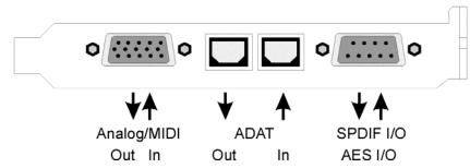
The **ADAT** I/O can also be used as **optical SPDIF** I/O, if set up accordingly in the Settings dialog.
