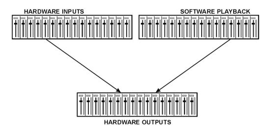
40 channels don't fit on the screen side by side, neither does such an arrangement provide a useful overview. The input channel should be placed above the corresponding output channel. Therefore, the channels have been arranged as known from an *Inline* desk, so that the row *Software Playback* equals the *Tape Return* of a real mixing desk:
