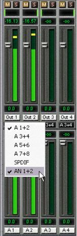
You will certainly have noticed that the signal at the outputs 7/8 did not change while you were routing channel 4 to other outputs and setting different gain values for those. With all analog and most digital mixing desks, the fader setting would affect the level for every routed bus - not so for TotalMix. TotalMix allows for setting all fader values individually. Therefore the faders and the panpots jump to the appropriate setting as soon as another routing is chosen.
