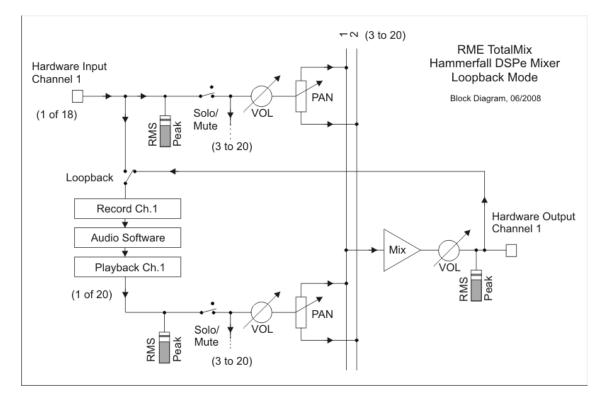
In loopback mode, the signal at the hardware input of the corresponding channel is no longer sent to the recording software, but still passed through to TotalMix. Therefore TotalMix can be used to route this input signal to any hardware output. Using the subgroup recording, the input can still be recorded on a different channel.
