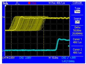
The cleaned and jitter-freed signal can be used as reference clock for any application. The signal processed by SteadyClock is not only used internally, but also available at the HDSPe AES word clock output. It is also used to clock the AES/EBU outputs.
