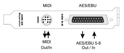
Note: If neither AES I/O 5-8 nor MIDI I/O is required, it is not necessary to install the Expansion Board at all.
