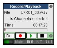
**Transport Bar.** Turning encoder 2 moves the cursor over *Del* (Delete), *Record*, *Play/Pause* and *Stop*. The selected function is initiated by pressing encoder 2. During playback the buttons Del / Record will change to Previous File / Next File.
