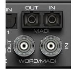
Selecting *Single Speed* in the Settings dialog causes the output signal to always stay within the range of 32 kHz to 48 kHz. So at 96 kHz and 192 kHz sample rate, the output word clock is 48 kHz.
