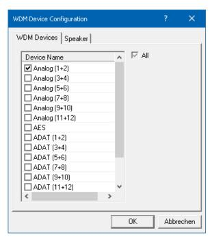
The screenshot to the left shows the multichannel WDM devices available with the UFX II after selecting 'Multi-Channel' in the WDM Devices listbox and hitting WDM Configure. In this example the devices Analog 1 to 8 and ADAT 1 to 8 are active.
