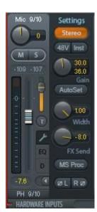
**AutoSet.** Activates an automatic gain reduction preventing overloads caused by too high gain settings. See chapter 19.2 for details.
