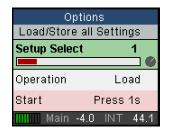
The Fireface UCX II can store and load its current state in 6 different memory slots, called Setups (SETUP/REV, Options, Load/Store all Settings). With this, the Fireface UCX II can be used stand-alone after setting it up accordingly, replacing lots of dedicated devices (see chapter 24).
