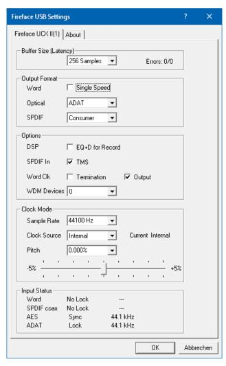
**TMS** activates the transmission of Channel Status data and Track Marker information on AES and SPDIF inputs. In case these information are not required the feature should be turned off.
