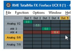
To maintain overview when the window size has been reduced, the labels are floating. They won't leave the visible area when scrolling. A right mouse click on the labels brings up the context menu with the exact same options as in the mixer view: Copy / Mirror / Paste /Clear input channels and submixes.
