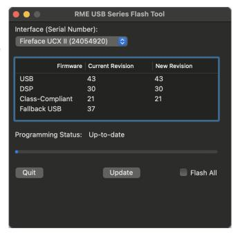
When the update fails (status: failure), the unit's second BIOS will be used from the next cold boot on (Secure BIOS Technology). Therefore the unit stays fully functional. The flash process should then be tried again on a different computer.
