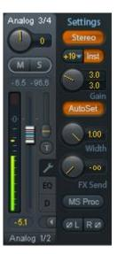
The instrument input operates unbalanced. Please don't use (stereo) TRS jacks in that mode.
