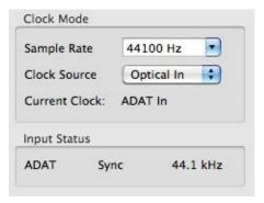
In practice, SyncCheck provides the user with an easy way of checking whether all digital devices connected to the system are properly configured. With SyncCheck, finally anyone can master this common source of error, previously one of the most complex issues in the digital studio world.
