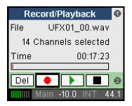
**Transport Bar.** Turning the encoder moves the cursor over *Del* (Delete), *Record*, *Play/Pause* and *Stop*. The selected function is initiated by pressing the encoder. During playback the buttons Del / Record will change to Previous File / Next File.
