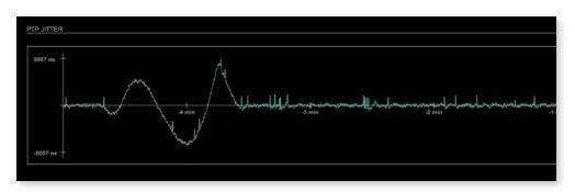
Graphical display of measured PTP jitter.
