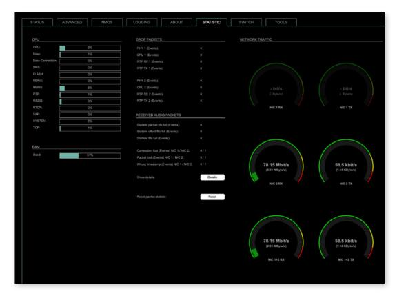
The tab 'STATISTIC' displays an overview of the CPU load of the particular processes, an error counter and a monitor display to indicate the incoming (RX) and outgoing (TX) network traffic on both network ports individually.
