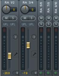
The **arrow symbol** at the bottom minimizes the channel width to that of the level meters. Another click maximizes it again. A mouse click with held Ctrl key causes all channels to the right to enlarge and minimize at once.
