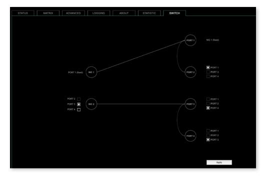
The device features four RJ45 sockets managed by two independent network interfaces (NIC 1 / NIC 2).
