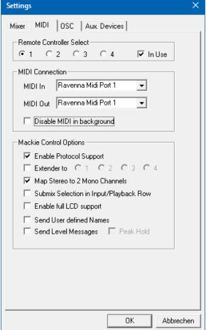
Note: When MIDI Out is set to NONE then TotalMix FX can still be controlled by Mackie Control MIDI commands, but the 8-channel block is not marked as remote target.
