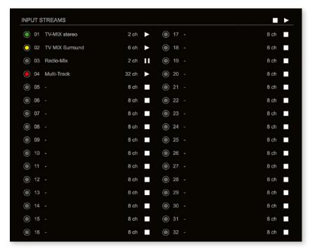
The module can subscribe up to 32 streams. The overview displays the basic information of each stream. The input stream name can be set manually (discovery protocol: manually, see page p 19) overriding the SDP's stream name information.
