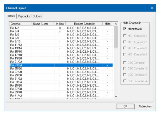
Hidden channels in *MIDI Remote x* are removed from the list of remote controllable channels. Within an 8-channel block of a Mackie compatible control they are skipped. The control therefore is no longer bound to consecutive orders. For example it will control channels 1, 2, and 5 to 11, when channels 3 and 4 are hidden.
