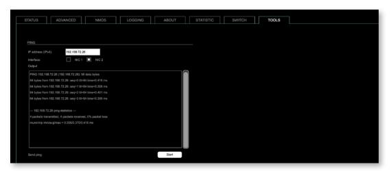
The tab 'TOOLS' offers a generator to ping any IP address (IPv4) from either NIC 1 or NIC 2. The result is displayed at the 'Output'.
