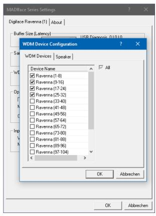
The screenshot to the left shows the multichannel WDM devices available with the Digiface Ravenna after selecting 'Multi-Channel' in the WDM Devices listbox and hitting WDM Configure. In this example the devices DRavenna 1-8, 9-16, 17-24 and 25-32 are active.
