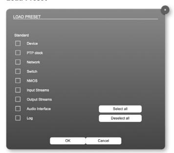
The device configuration can be stored to a single file (.rps).
