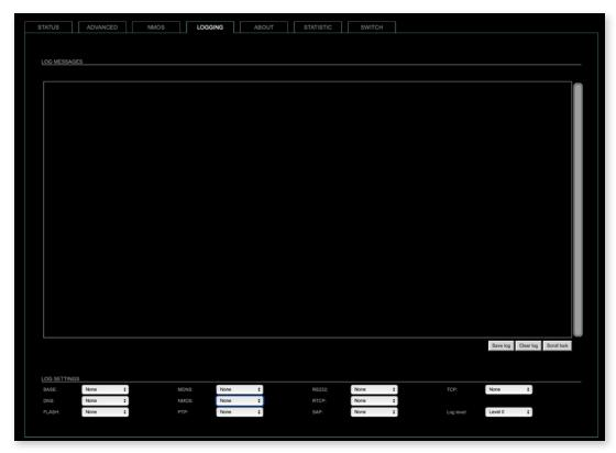
The tab 'LOGGING' displays logging depending on the 'Log Settings'. The logging can be enabled individually for different protocols, each of with an adjustable filter. An adjustable log level specifies the information detail of each entry.
