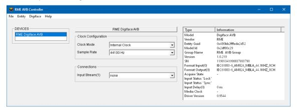
The screenshot shows the basic functions of the AVB Controller, which appear as soon as a network cable is plugged into the Gigabit ethernet port of the Digiface AVB. In case this is not an AVB network no other AVB devices are shown, but the Digiface AVB itself is displayed and the sample rate is now selectable.
