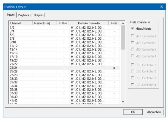
Hidden channels in *MIDI Remote x* are removed from the list of remote controllable channels. Within an 8-channel block of a Mackie compatible control they are skipped. The control therefore is no longer bound to consecutive orders. For example it will control channels 1, 2, and 5 to 10, when channels 3 and 4 are hidden. The same can be done for OSC. With unnecessary channels made invisible for the OSC remote the more important channels are available as one block on the remote.
