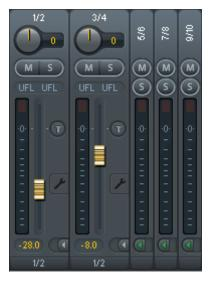
The **arrow symbol** at the bottom minimizes the channel width to that of the level meters. Another click maximizes it again. A mouse click with held Ctrl key causes all channels to the right to enlarge and minimize at once.
