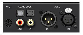
MIDI I/O. Two 5-pin DIN connectors provide MIDI input and output.
