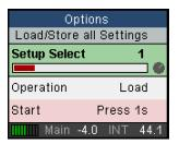
The Digiface AES can store and load its current state in 6 different memory slots, called Setups (SETUP/REV, Options, Load/Store all Settings). With this, the Digiface AES can be used stand-alone after setting it up accordingly, replacing lots of dedicated devices (see chapter 24).
