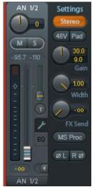
Input channels 3 and 4 are found as TS jacks on the right side of the Babyface Pro. These Hi-Z **universal inputs** have an input impedance of 1 MOhm. The input gain is controlled and performed digitally and limited to 9 dB. An additional hardware-based reference level optimizes the signal to noise ratio. Choices are +4 dBu and -10 dBV.
