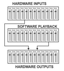
Click on the Hardware Output channel in the third row where the audio signal is supposed to show up. This channel turns brighter, means it is selected as current submix. Now move the faders up from all sources – these are the input and playback channels, in the first and second row. That's it. The input (monitoring) and playback (DAW software) audio signals are now available at that very output, which can be verified immediately from the level meters reacting accordingly.
