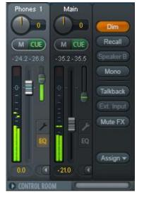
**Speaker B.** Switches audio from Main Out to Main Out B. The faders of the channels Main and Speaker B can be ganged via Link. Via *Options / Key Commands* switching to Speaker B can also be controlled by the unit's **OUT**, **A**, **B** and **DIM** button.
