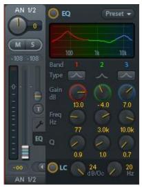
The frequency graphics give a precise overview of the filter results. Overlapping filters influence each other. This can be used to achieve more than 20 dB amplitude, or to generate difficult frequency response optimizations.
