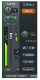
Loopback. Sends the output data to the driver as record data. The corresponding submix can
