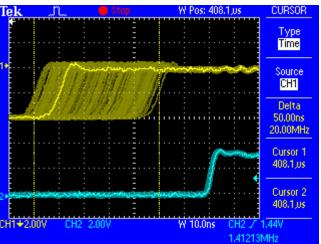
The screenshot shows an extremely jittery SPDIF signal of about 50 ns jitter (top graph, yellow). SteadyClock turns this signal into a clock with less than 2 ns jitter (lower graph, blue). The signal processed by SteadyClock is of course not only used internally, but also used to clock the digital output. Therefore the refreshed and jitter-cleaned signal can be used as reference clock without hesitation.
