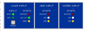
In the AES INPUT STATE section, each of the 32 inputs has its own SYNC LED. One LED per (stereo) input indicates audio information within the data stream. An input signal in the range of 60 kHz to 100 kHz will turn the DS LED on. An input signal in the range of 162 kHz to 200 kHz will turn the QS LED on.
