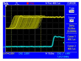
The cleaned and jitter-freed signal can be used as reference clock for any application, without any problem. The signal processed by SteadyClock is of course not only used internally, but also available at the ADI-6432's word clock output. It is also used to clock the digital outputs MADI and AES.
