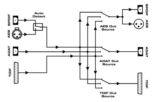
The three input formats AES/SPDIF, ADAT and TDIF on the left side are sent to three *Output Source* selectors each. Using these selectors, the three outputs on the right side gain access to any of the three inputs. As all three selectors operate independently, all three outputs can even use the same input signal, so AES is converted to AES, TDIF and ADAT at the same time – just an example. Any combination that one can imagine is allowed.
