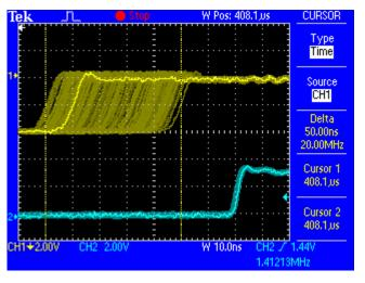
The cleaned and jitter-freed signal can be used as reference clock for any application, without any problem. The signal processed by SteadyClock is of course not only used internally, but also available at the ADI-192 DD's word clock output. It is also used to clock all the digital outputs.
