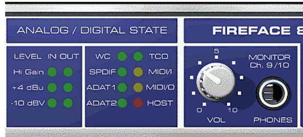
The red **HOST** LED lights up when the Fireface 800 has been switched on, signalling the presence of operating voltage. At the same time it operates as error LED, in case the FireWire connection hasn't been initialised yet, or has been interrupted (error, cable not connected etc.).
