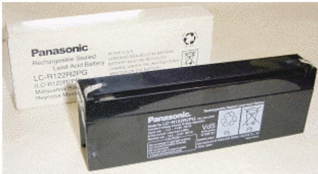
We tested a Panasonic LC-R122R2PG battery, 12 V 2.2 Ah, which can operate the QuadMic for 4 hours. Measuring the voltage while discharging shows that the QuadMic remains completely in working order even shortly before the battery collapses (6 Volts.)
