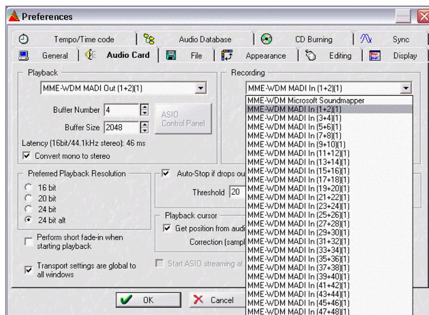
The HDSP MADI allows sample rates of up to 96 kHz via MADI. In this mode, only channels 1 to 32 are available.
