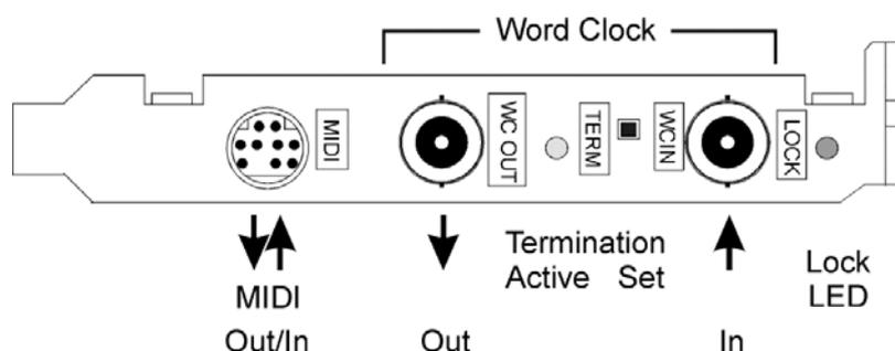
The included breakout cable is connected to the **9-pin Mini-DIN** connector and provides **two MIDI** inputs and outputs via four **5-pin DIN** connectors.
