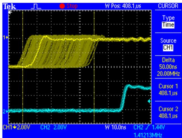
The cleaned and jitter-freed signal can be used as reference clock for any application, without any problem. The signal processed by SteadyClock is of course not only used internally, but also available at the HDSP MADI 's word clock outputs. It is also used to clock the digital MADI output.
