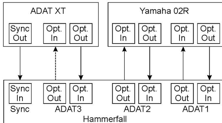
Because the ADAT recorder is not receiving any signal from HDSP or from the mixer, it will generate its own clock at a rate which is (almost) the same as the sample frequency of the mixing desk - but not identical.
