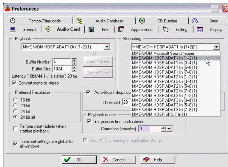
The HDSP system's ADAT optical interface allows sample rates of up to 96 kHz using a standard ADAT recorder. Single-channel data at this frequency requires two ADAT channels, achieved using the *Sample Multiplexing* technique. This reduces the number of available ADAT channels from 8 to 4 per ADAT port. Under Windows MME, channels are routed to ADAT devices in double-speed mode as follows:
