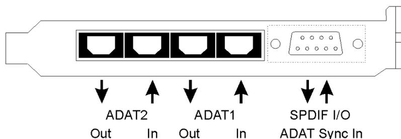
The **ADAT1** I/O next to the D-type socket can also be used as **optical SPDIF** I/O, if set up accordingly in the Settings dialog.
