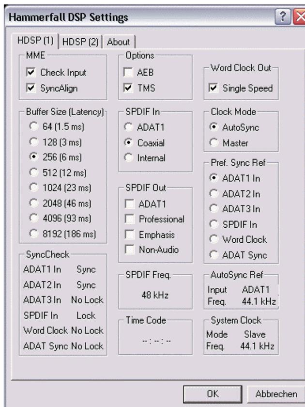
*SyncCheck* indicates whether there is a valid signal (Lock, No Lock) for each input (Word Clock, ADAT 1-3, SPDIF, ADAT Sync), or if there is a valid *and* synchronous signal (Sync). The *AutoSync Ref(erence)* display shows the input and frequency of the current sync source.
