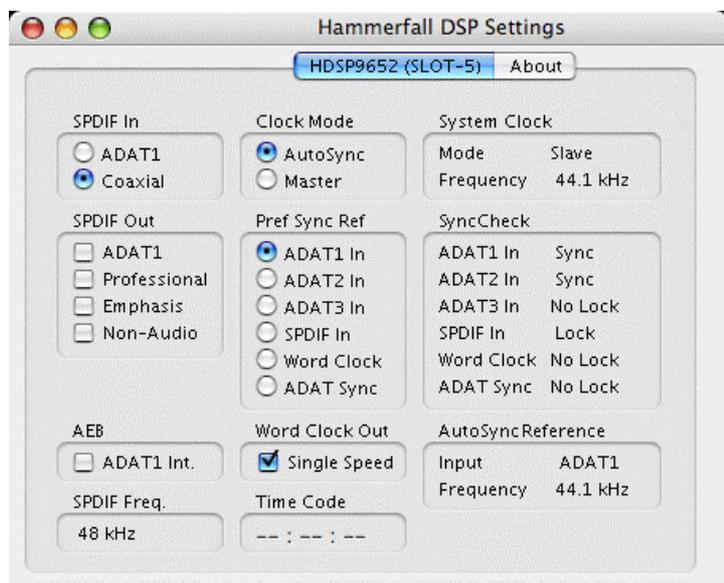
If several digital devices are to be used simultaneously in a system, they not only have to operate with the same sample frequency but also be synchronous with each other. This is why digital systems always need a single device defined as 'master', which sends the same clock signal to all the other ('slave') devices.
