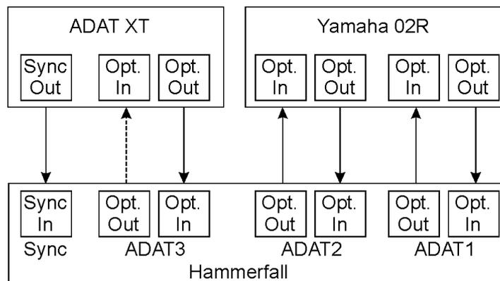
Remedy: To drive the ADAT recorder from its digital input, set it to slave mode (DIG), and connect the input to the HDSP's ADAT3 output. The Hammerfall DSP is already in sync with the mixing desk, so it will send an identical (synchronous) signal to ADAT3 out. The ADAT recorder will lock onto this, its output will also be in sync. The signal from the ADAT recorder is now fully in sync with the signals from the mixing desk.
