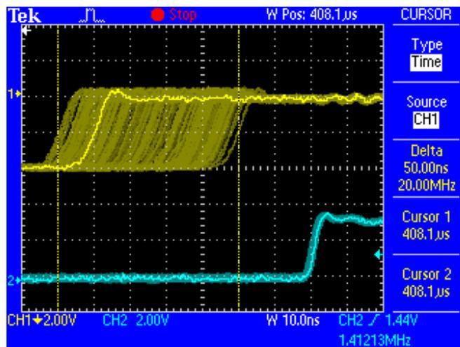
The screenshot shows an extremely jittery SPDIF signal of about 50 ns jitter (top graph, yellow). Thanks to SteadyClock this signal turns into a clock with less than 2 ns jitter (lower graph, blue). The signal processed by SteadyClock is of course not only used internally, but also used to clock the digital outputs. Therefore the refreshed and jitter-cleaned signal can be used as reference clock without hesitation.
