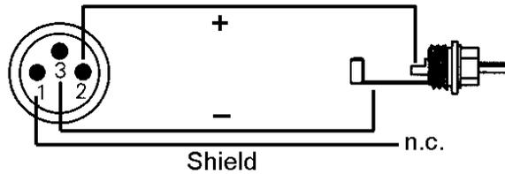
Using this cable adapter XLR/RCA devices with coaxial SPDIF interface can be connected to the AES output of the RayDAT as well. Note that most consumer equipment with RCA SPDIF inputs will only accept signals having a Channel Status *Consumer*. In such cases the above adapter cable will not work.
