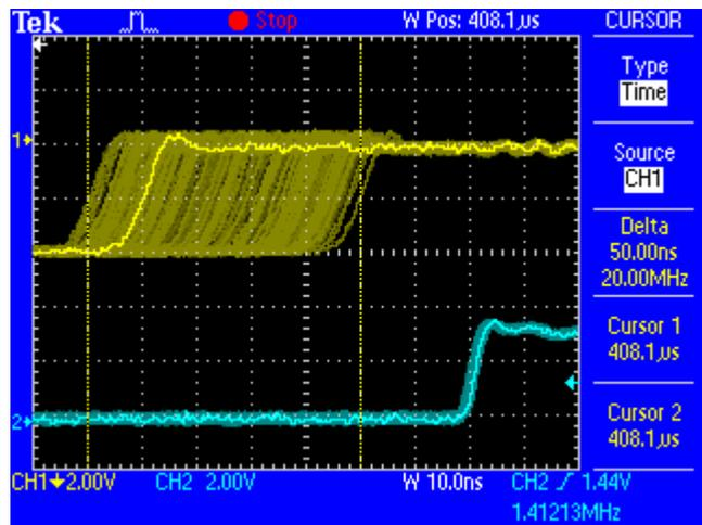
The cleaned and jitter-freed signal can be used as reference clock for any application. The signal processed by SteadyClock is not only used internally, but also available at all outputs of the HDSPe RayDAT.
