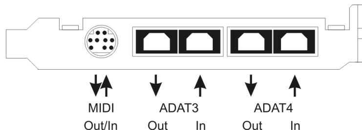
**ADAT4** can also be used as **optical SPDIF I/O**, if set up accordingly in the Settings dialog.
