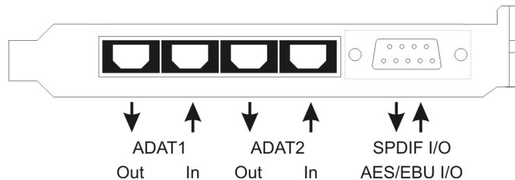
The Expansion Board's bracket gives access to a **third and fourth ADAT optical** input and output.
