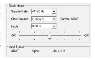
This way, configuring any suitable audio application for digital recording is simple. After selecting the required input, Fireface 400 displays the current sample frequency. This parameter can then be changed in the application's audio attributes (or similar) dialog.
