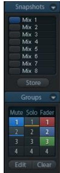
TotalMix uses flashing signals to guide you through the group setup. After a click on Edit and click on the desired storage place all desired functions for this group have to be activated or selected. The storage process is finished by another click on Edit.
