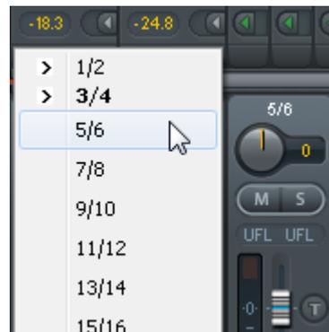
An arrow is only shown with an activated routing. A routing is seen as activated when audio data is sent. As long as the fader is set to  $-\infty$  the current routing will be shown in bold letters, but not have an arrow in the front.
