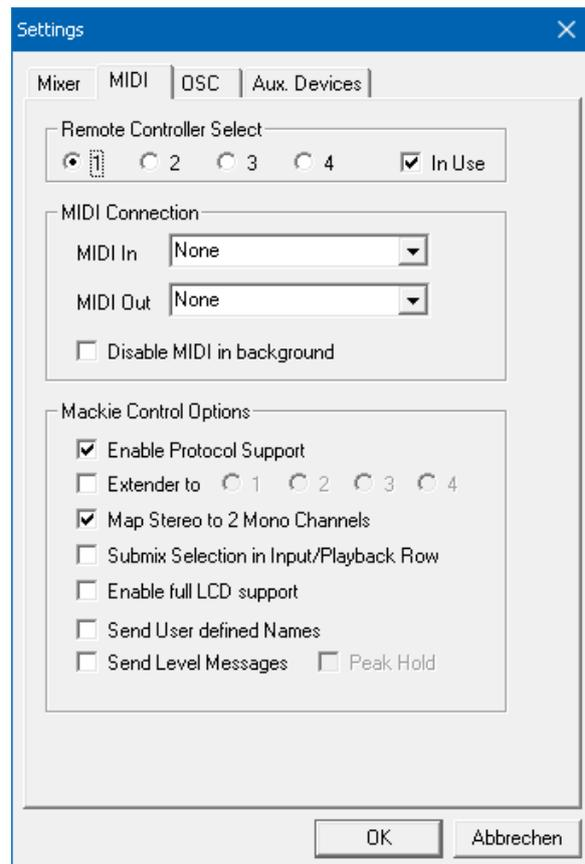
Note: When MIDI Out is set to NONE then TotalMix FX can still be controlled by Mackie Control MIDI commands, but the 8-channel block is not marked as remote target.
