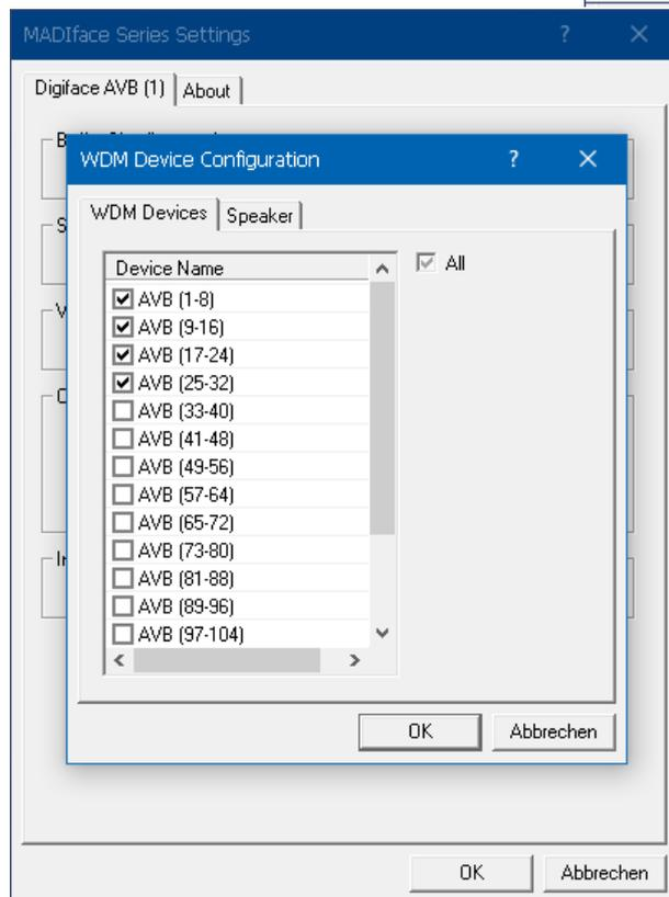
The screenshot to the left shows the multi-channel WDM devices available with the Digiface AVB after selecting 'Multi-Channel' in the WDM Devices listbox and hitting *WDM Configure*. In this example the devices AVB 1-8, 9-16, 17-24 and 25-32 are active.
