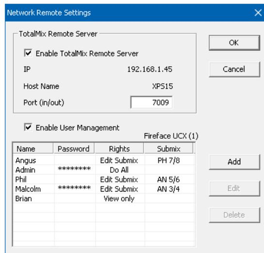
Tap Done on top or click Ok. In the mixer view the state should change from *offline* to *connected* within a few seconds.
