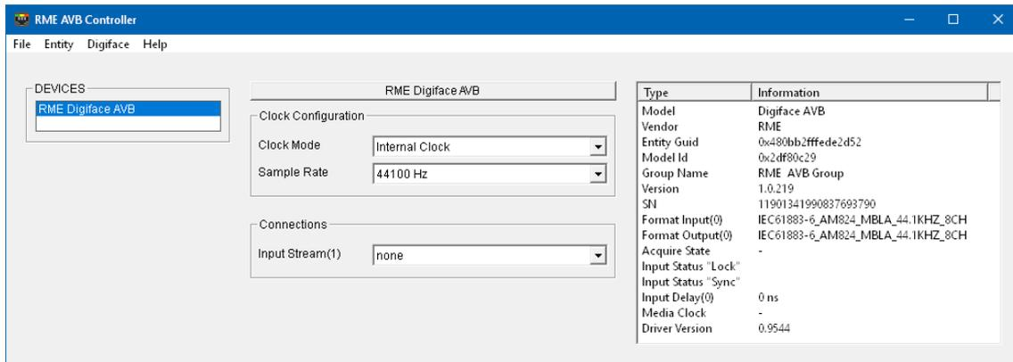
The screenshot shows the basic functions of the AVB Controller, which appear as soon as a network cable is plugged into the Gigabit ethernet port of the Digiface AVB. In case this is not an AVB network no other AVB devices are shown, but the Digiface AVB itself is displayed and the sample rate is now selectable.
