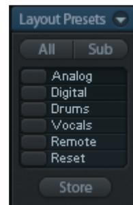
With a simple click on a button it will then be possible to easily switch views of only the channels involved with the mixing of the drum section, the horn section, the violins, or any other useful view. An optimized remote layout can be activated here as well, with or without visible changes. Double-click the default slot name to enter any other name.
