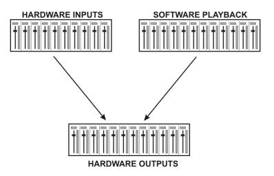
TotalMix can be used in the above view (View Options **2** Rows). However, the default is a vertical alignment in three rows as known from an Inline desk, so that the row *Software Playback* equals the *Tape Return* of a real mixing desk:
