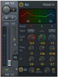
**Preset.** Settings of the EQ and the Low Cut can be stored, loaded, and copied between channels at any time. A click on Preset opens a menu with several entries:
