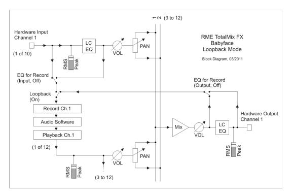
The block diagram shows how the software's input signal is played back, and fed back from the Hardware Output to the software input.
