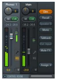
**Speaker B.** Switches playback from Main Out to Main Out B. The faders of the channels Main and Speaker B can be ganged via Link. Via *Options / Key Commands* switching to Speaker B can also be controlled by the unit's **Select** button.
