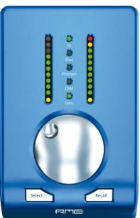
The key **Recall** is used to store and load a specific listening volume for the Main Out (default: Analog 1/2) defined in TotalMix FX. Pushing the knob for 2 seconds stores the current setting. If the volume (output level) had been changed a quick hit on the Recall key will restore the former value.
