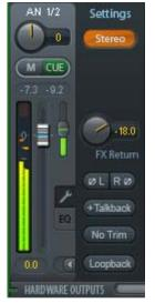
**Loopback.** Sends the output data to the driver as record data. The corresponding submix can be recorded then. This channel's hardware input sends its data only to TotalMix, no longer to the recording software.
