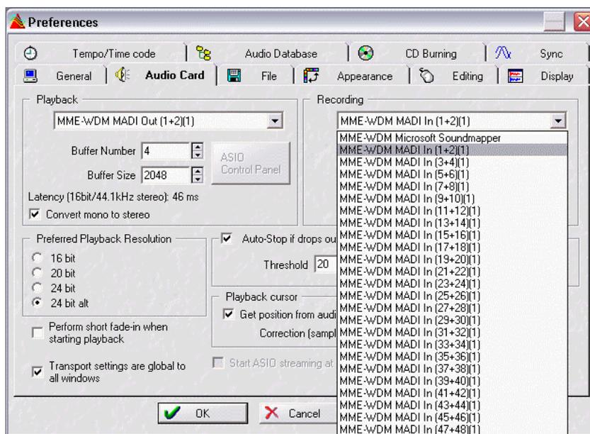
The MADiface allows sample rates of up to 192 kHz via MADi. In this mode, only channels 1 to 16 are available.
