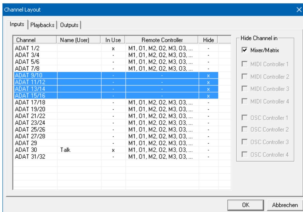
Hidden channels in *MIDI Remote* *x* are removed from the list of remote controllable channels. Within an 8-channel block of a Mackie compatible control they are skipped. The control therefore is no longer bound to consecutive orders. For example it will control channels 1, 2, and 5 to 10, when channels 3 and 4 are hidden.
