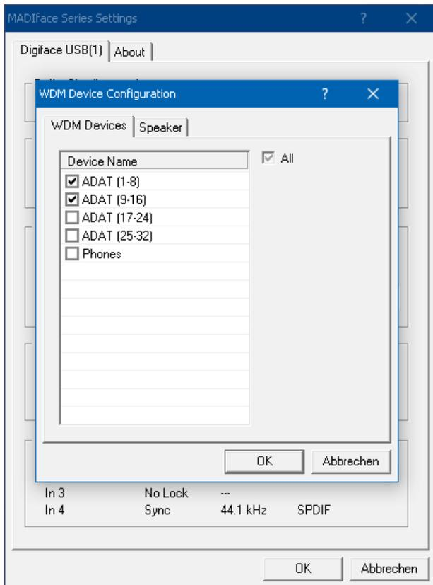
The screenshot to the left shows the multi-channel WDM devices available with the Digiface USB after selecting 'Multi-Channel' in the WDM Devices listbox and hitting *WDM Configure*. In this example the devices *ADAT 1 to 8* and *ADAT 9 to 16* are active.
