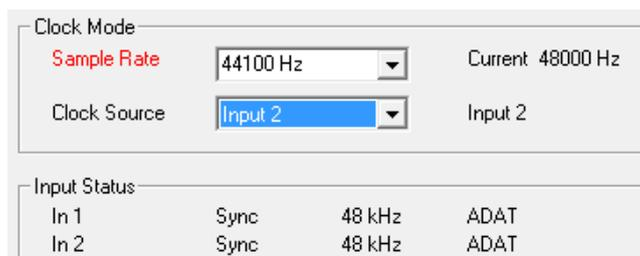
Under ASIO the audio software sets the sample rate, so that such an error can not happen. If the input sample rate is different then there will be no Sync indication.
