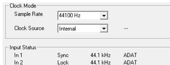
This way, configuring any suitable audio application for digital recording is simple. After connection the Digiface USB displays the current and external sample frequency. This parameter can then be changed in the application's audio attributes (or similar) dialog.
