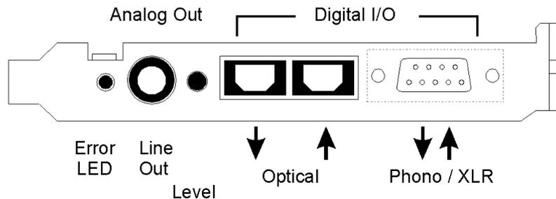
All outputs are driven in parallel, therefore carrying identical signals. In the simplest situation, connect 3 devices at the outputs and use the card as a splitter (distribution 1 to 3).
