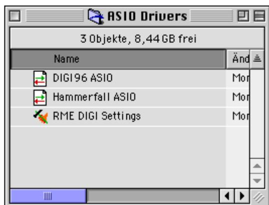
Copy the new files **RME DIGI Settings** and **Hammerfall ASIO** into all 'ASIO Drivers' folders found on your computer. As every ASIO software has its own ASIO Drivers folder the files have to be copied several times. The picture to the left shows an example after installation of Hammerfall and DIGI96.
